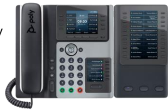
Monitor up to 66 additional lines by adding 1 Poly Edge E Expansion Module
